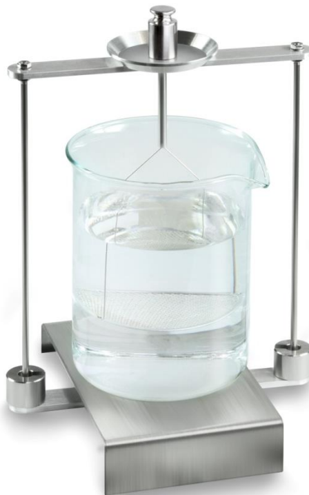
Fig.1: Weighing in air The weight of the „sample in air“ is displayed.
