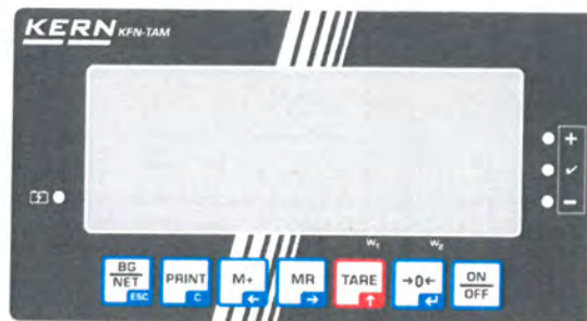
Figure 2 Indicator front layout for KFN-TAM / BFA...AM / BFN...AM / SFB...AM / NFN...AM / NBB...AM / UFN...AM / UFC...AM
