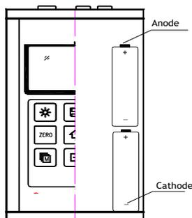
If the unit is not used for a long period of time, the batteries should be removed. It is recommended to replace the batteries already when the capacity is down to 10%.
