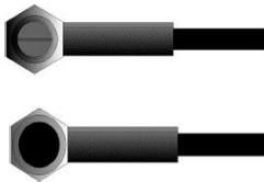
The upper figure shows the bottom view of a typical measuring probe. The two half circles are visible, visibly divided in the middle. One of the semicircles directs the ultrasound into the material to be measured and the other directs the echo back to the measuring probe. When the measuring probe is placed on the material to be measured, it is located directly under the centre of the spot whose thickness is to be measured.
