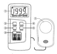
1st LCD display: 3 ½ digits with maximum reading value until 1999.
