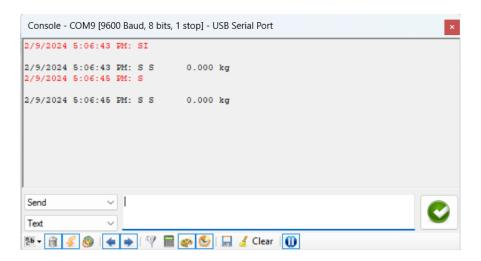
The terminal displays the data received from the connected device and the data transmitted to the device by the software as raw data. In the toolbar you can choose between a variety of display options.
