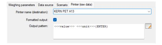
This allows, for example, to format a scale output in a particular way and forward it to a printer. Special functions for ZPL2 printers allow to use images or rendered PC fonts with compatible printers.
