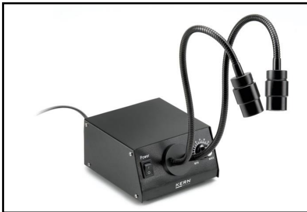
Typical goose neck lighting unit
