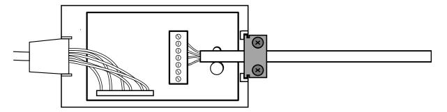
**8.** Clip the upper half of the module enclosure back on.
