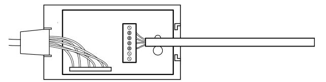
**6.** Insert the lower part of the cable gland into the guide of the module enclosure and place the cable into the cable gland.
