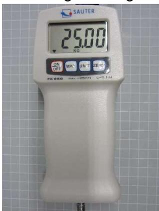
4. The corresponding weight is now attached to the hook. The device **must be held still while the weight is attached**; avoid shaking. Tip: hold the device with both hands while resting both elbows on a table or attach it to a fixed object (test stand).
