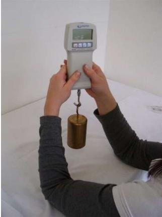
5. This position is held until **"F"** appears on the display. The weight can then be removed and the adjustment is complete. However, if **"E"** appears on the display, repeat steps 1 to 5 until a successful adjustment is confirmed with **"F"**.
