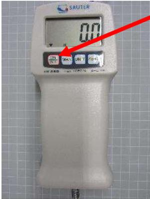
2. As soon as "0" appears on the display, press the **"UNIT"** button and the **"ZERO"** button simultaneously until **"CAL"** appears on the display.
