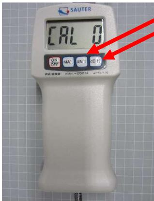
3. After a few seconds, the required **calibration weight** appears on the display, e.g. 5.00 kg for the FK 50 or 10.00 kg for the FK 100.
