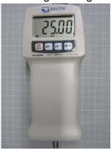
4. The corresponding weight is now attached to the hook. The device **must be held still while the weight is attached**; avoid shaking. <u>Tip:</u> hold the device with both hands while resting both elbows on a table or attach it to a fixed object (test stand).
