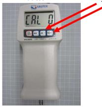
3. After a few seconds, the required **calibration weight** appears on the display, e.g. 5.00 kg for the FK 50 or 10.00 kg for the FK 100.
