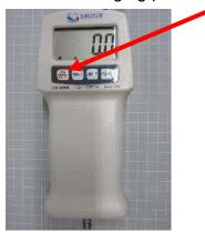
2. As soon as "0" appears on the display, press the **"UNIT"** button and the **"ZERO" button** simultaneously until **"CAL"** appears on the display.
