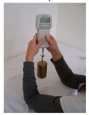
5. This position is held until **"F" appears on** the display. The weight can then be removed and the adjustment is complete. However, if **"E" appears on the display**, repeat steps **1** to **5 until** a successful adjustment is confirmed with **"F"**.
