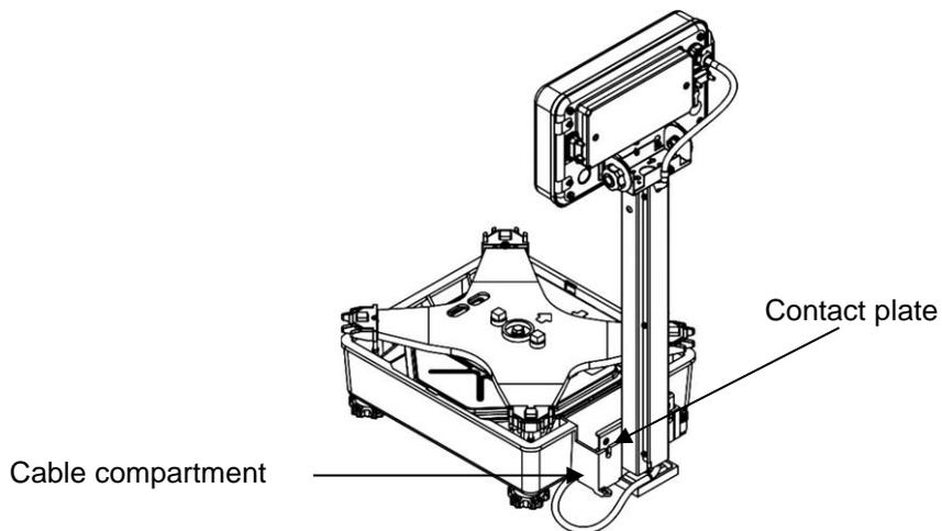
8. Pull the scale cable [5] through the lower recess of the stand [2].
