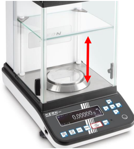
Fig.1 Internal windshield with long carriers.
