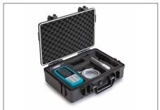
Scope of delivery: Standard block for calibration (approx. 61 HRC), USB cable, display unit, UCI sensor unit, transport case, software to transfer the saved data to the PC, other accessories
